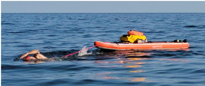
Fig. 5: eSUP (electric Stand-Up Paddleboard) as a towfloat to help a swimmer pull (tow) a heavy load. Assist from motors mounted to fins (underwater and therefore not visible in photo) is used to maintain a constant tension in the tether and alleviate force required to tow the paddleboard.
