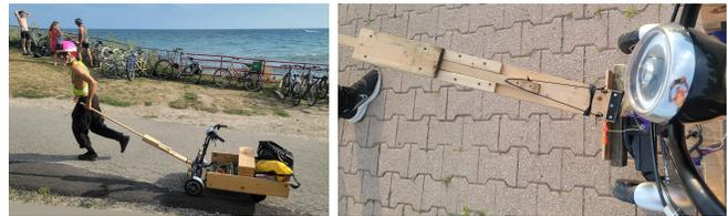
Fig. 12: The Freehicle is a vehicle for freedom of mobility. A person can ride on it or pull it like a wagon.
