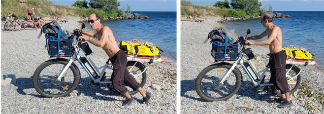
Fig. 9: Cybernetic control of electric cargo bicycle while pushing it up a steep incline on a pebble beach, loaded with paddleboard, safety equipment, drybag of food, and other provisions, etc.. (Left) without cybernetic assist; (Right) with cybernetic assist.
