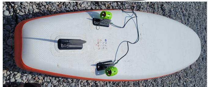
Fig. 3: Bottom view of paddleboard. Thrusters provide support to paddler in proportion to paddle flex, or to swimmer in proportion to force exerted on a tow cord / cable.
